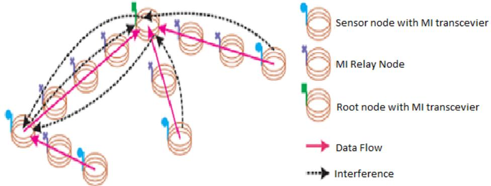
**Figure 2: MI Relay based transmission**
