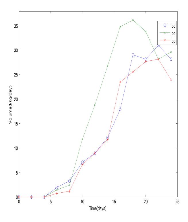
Figure 1: Daily gas yield during batch digestion of 3 categories of wastes. pc-poultry dropping and cassava peelings and water. bc-beans waste and cassava peelings and water. pb-poultry droppings and beans waste and water.
