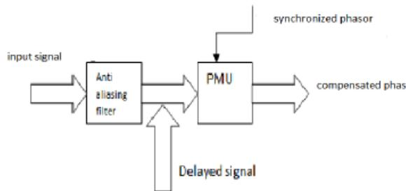
Fig.4 Compensating for signal delay introduced by the anti aliasing filter.
