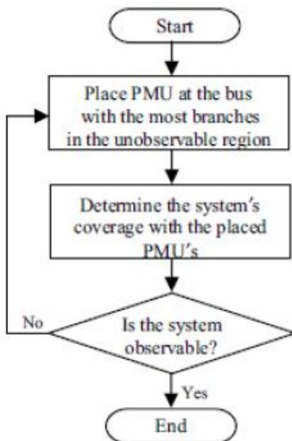
Fig. 6. Flowchart of the Graph Theoretic Procedure
