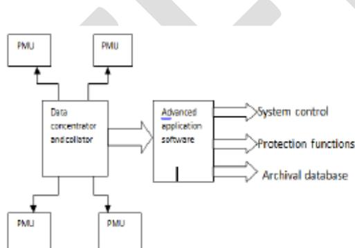
Fig.3 PMU utilization in a power system
