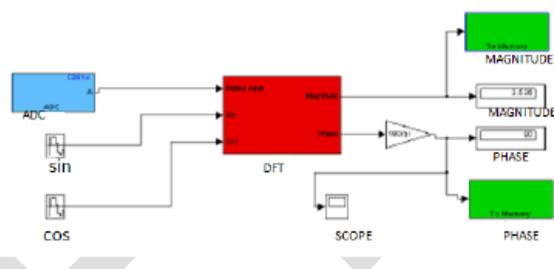
Fig.1 phasor measurement for single phase analog input
