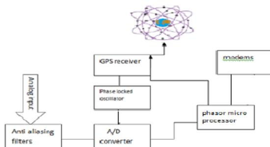
Fig.2 General Block Diagram of PMU
