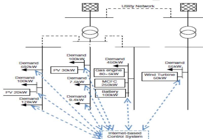
Fig. 2. Kyoto Eco-Energy virtual microgrid schematic diagram [5]
