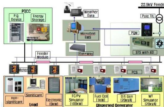
Fig 7 KERI microgrid pilot plant system configuration [13]
