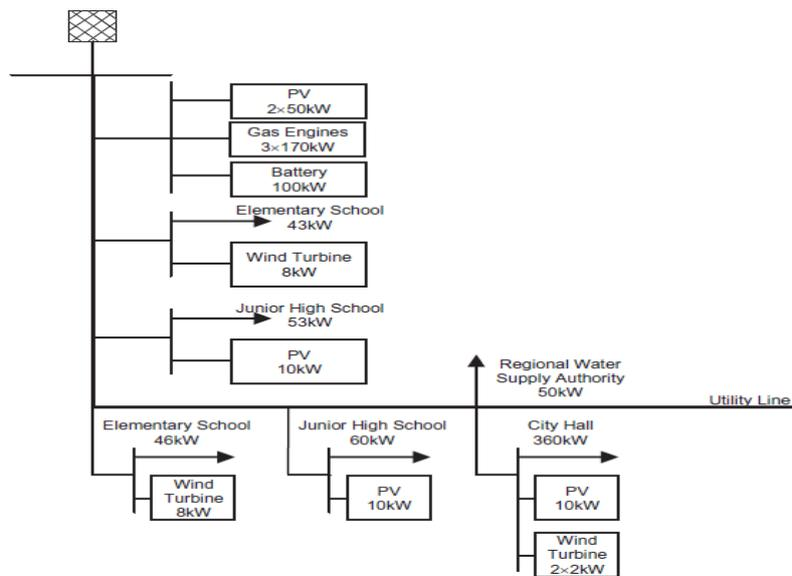
Fig. 3. The schematic diagram of the Hachinohe microgrid [5]
