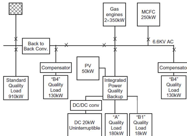
Fig 4. The schematic diagram of the Sendai microgrid [5]
