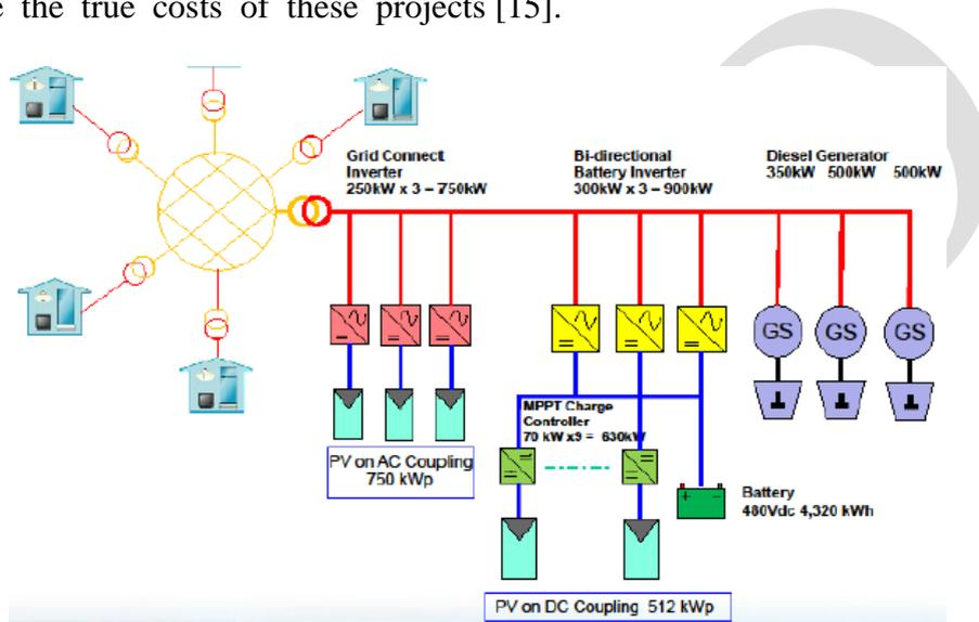
Fig 9 MW Scale System Tanjung Labian, Sabah (Malaysia)[15]
