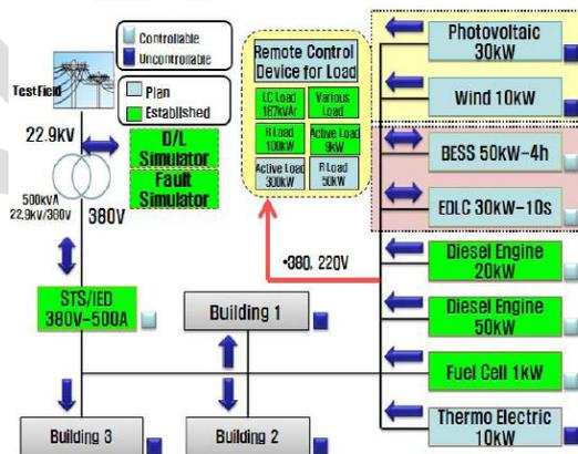
Fig. 8 KERI's future microgrid pilot plant system [14]
