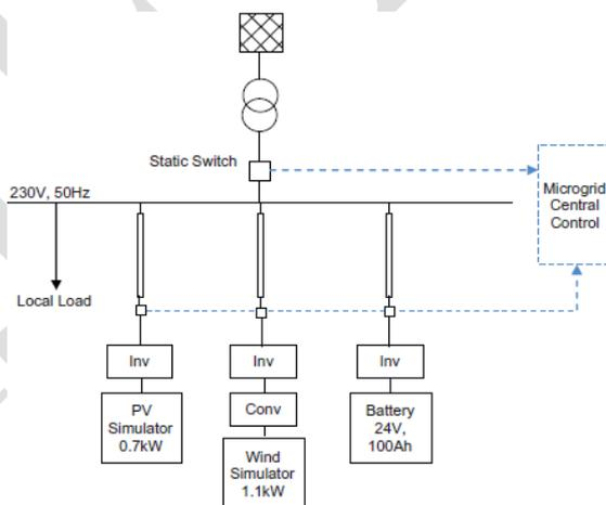
Fig.6 . Laboratory scale microgrid in Hong Kong [12]
