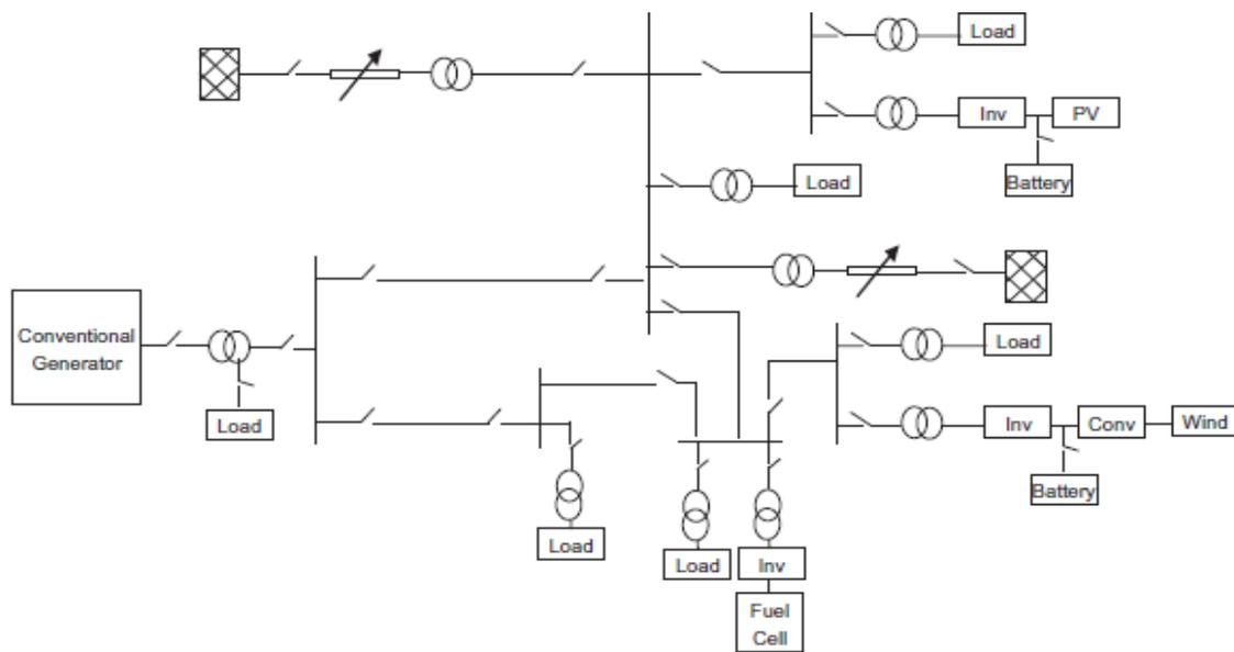
Fig 5. Microgrid testbed in Hefei University of Technology [11]
