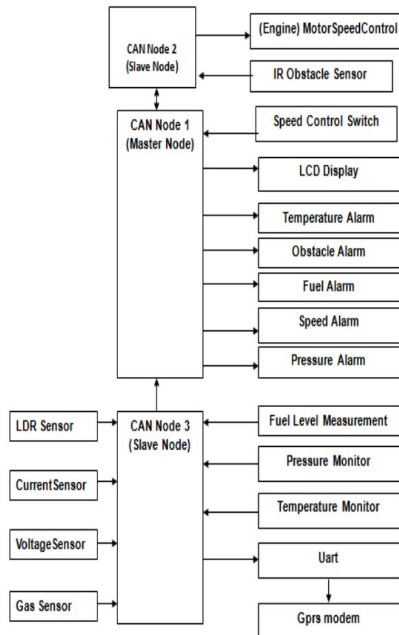
Fig 1: BLOCK DIAGRAM
