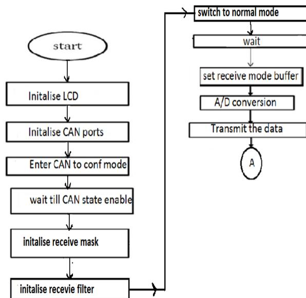
Fig 3: flow chart for can based monitoring system
