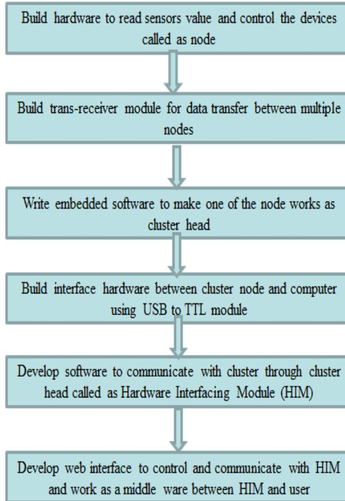
Figure 3: Flow Diagram
