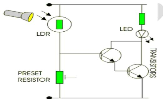
**Fig. 5.4** LED based LDR Sensor
