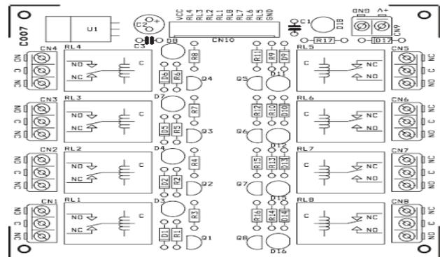
**Fig. 5.4** Eight relay circuit diagram with ULN driver
