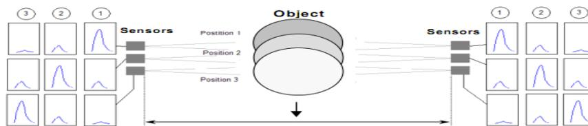
Fig. 1. Basic configuration of the detector and amplitudes of the output signals for different object positions 1, 2, 3 (left and right columns), illustrating the working principle
