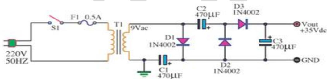
Fig 5.9 Voltage convertor circuit
