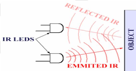
Fig 5.6 I.R. Sensing logic
