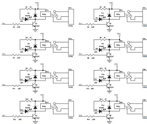
**Fig. 5.3** Eight Relays Circuit
