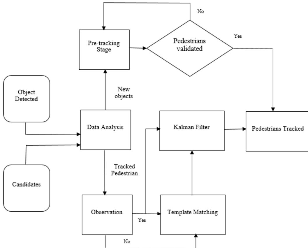
Fig 8: Tracking Module
