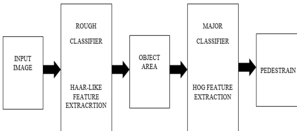
Fig 4: Two Stage Object classifier
