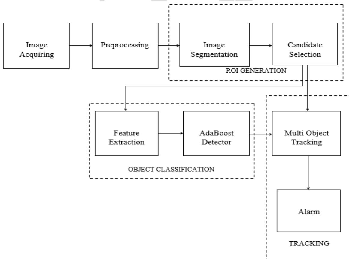
Fig 3: Pedestrian Detection System
