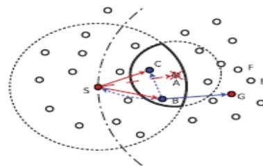
Fig 4.3 Handling the best forwarder failure
