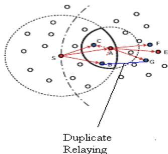
Fig 4.4 Link failure between Forwarding candidate and best forwarder
