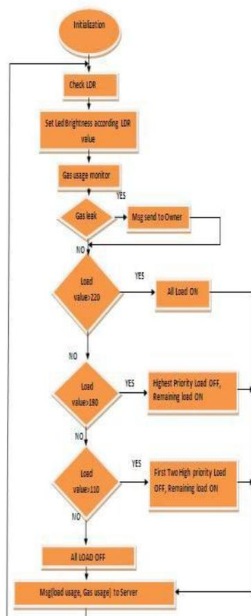
**Fig. 3 System Flow Diagram for the Proposed System**
