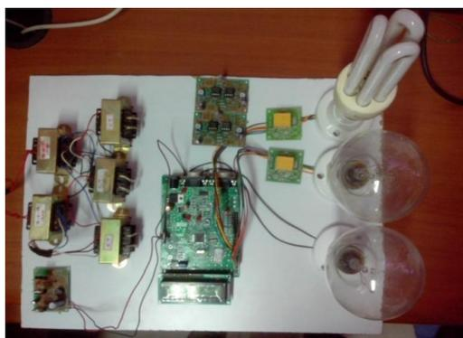
**Fig. 7 Experimental Setup for the Load Priority System**
