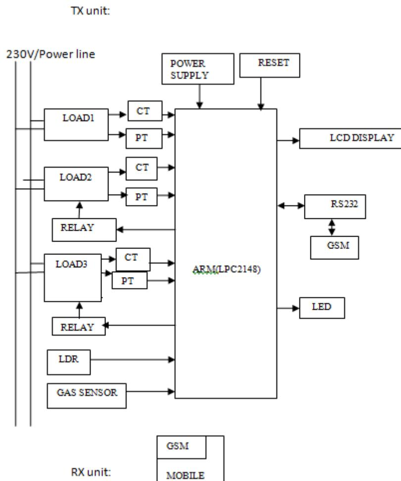
**Fig. 2 Block Diagram of the Proposed System**
