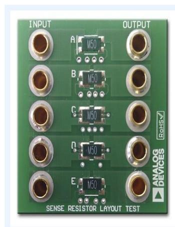
Fig 4: Sense resistor layout test PCB.
