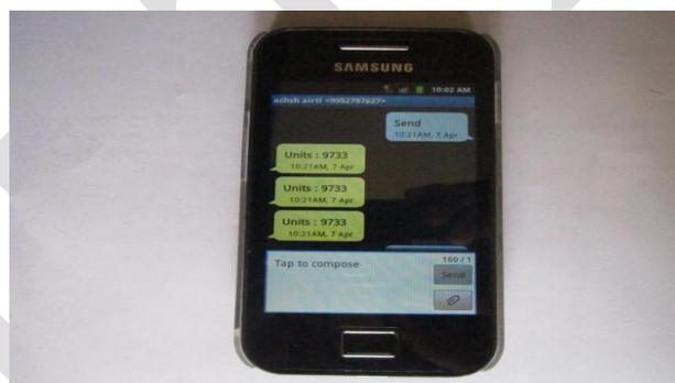
Fig 11: Snap shot of reading received by the consumer
