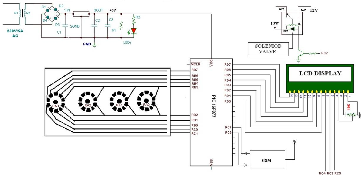
Fig 6: Hardware Circuit Diagram
