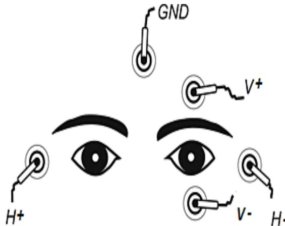
Figure 2: Placement of electrodes
