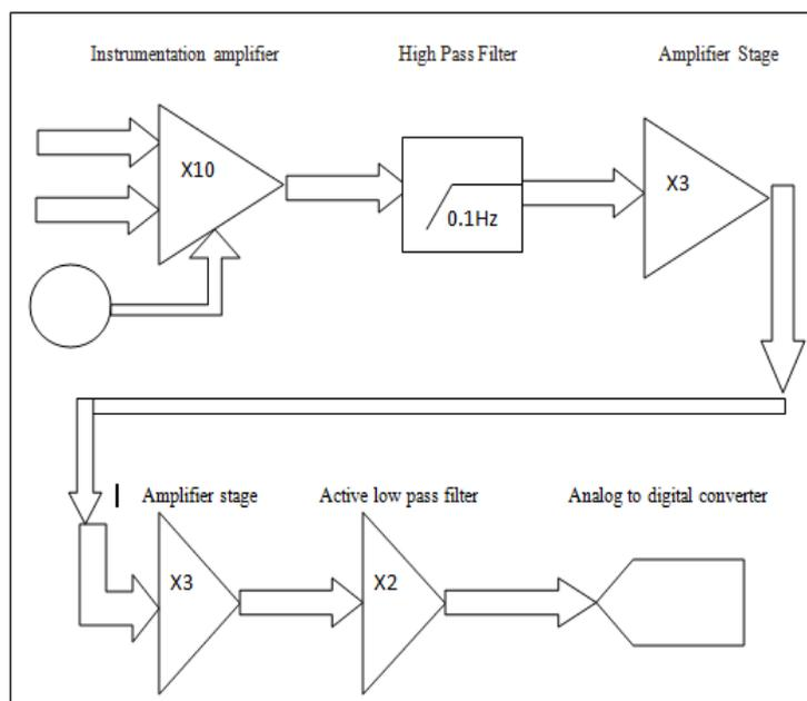
Figure 3: Block diagram of proposed system
