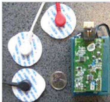
Figure 5: Electrodes with AVR processor
