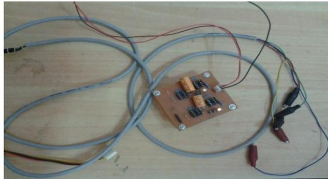
Figure 6: Designed stereo amplification circuit with connecting cables which is responsible for the amplification of left and right movement of eyes
