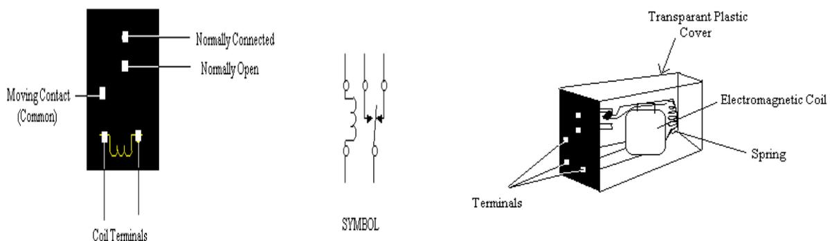
**Fig.7** Structure of Relay and Its Symbol
