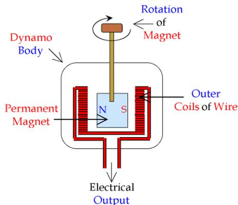
**Fig.4** Working of Dynamo
