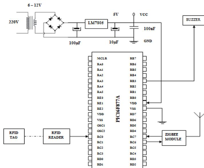
**Figure 7. Circuit Diagram of the Receiving Section**
