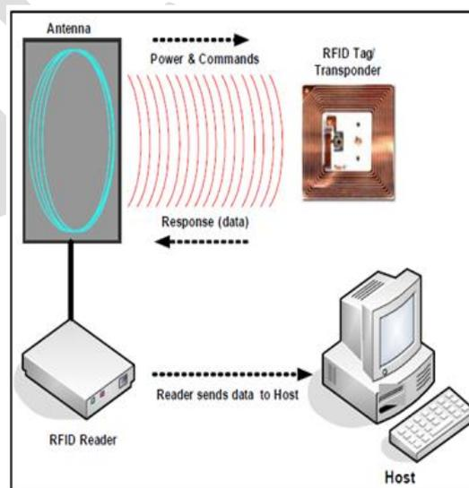
Figure 1. Typical RFID System
