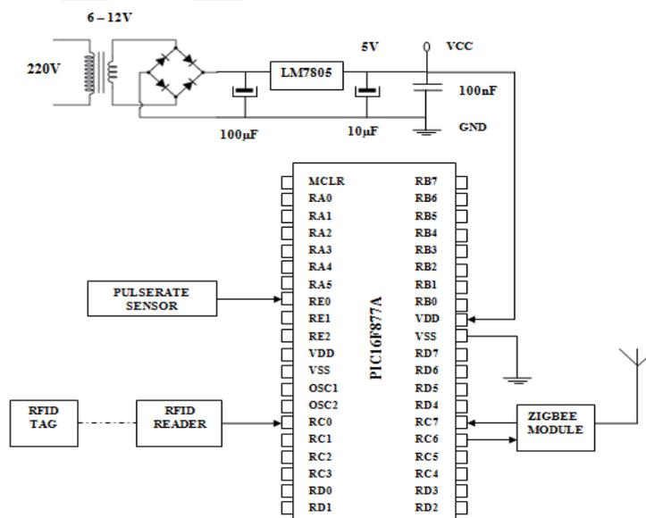
**Figure 6 Circuit Diagram of the Transmitting Section**
