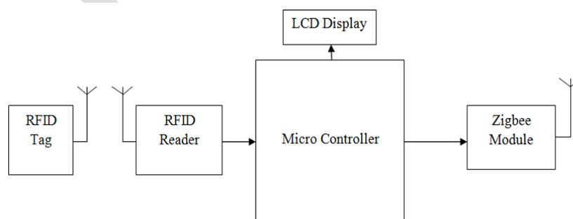
**Figure 4. Block Diagram of the Readers Unit**
