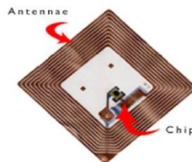
**Figure 2. Components of RFID Tag**
