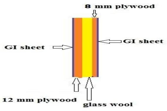
**Fig1 Cross section of chamber wall**
