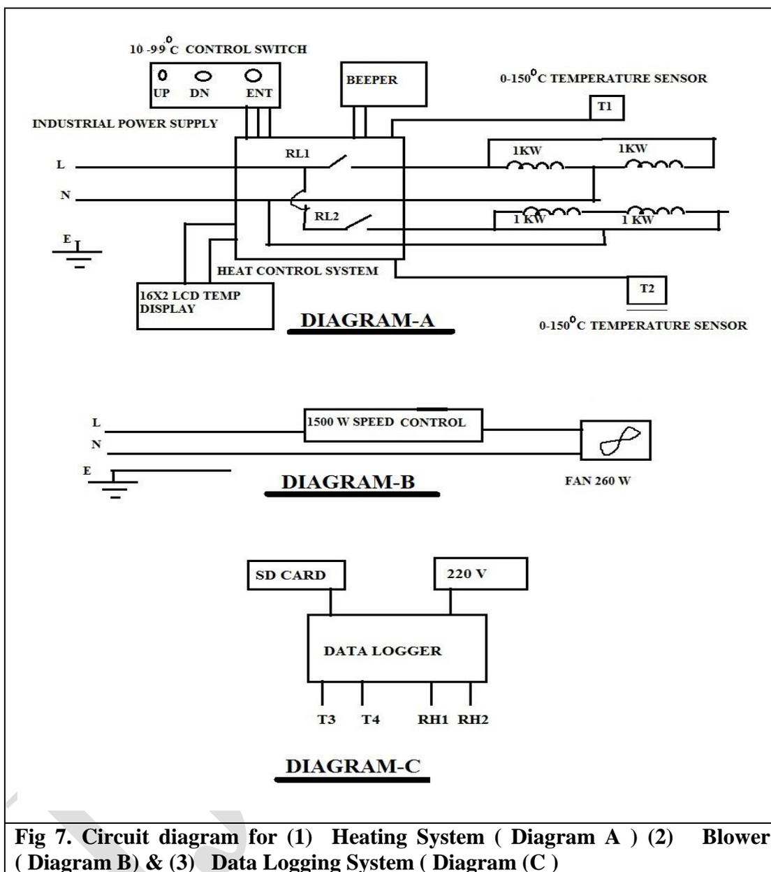
**Fig 7. Circuit diagram for (1) Heating System ( Diagram A ) (2) Blower ( Diagram B ) & (3) Data Logging System ( Diagram ( C )**
