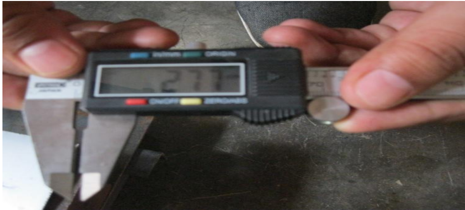
Figure.4. digital reading of sheet metal
