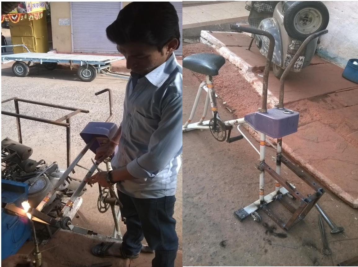
Fig.3. Construction of Work piece Frame
