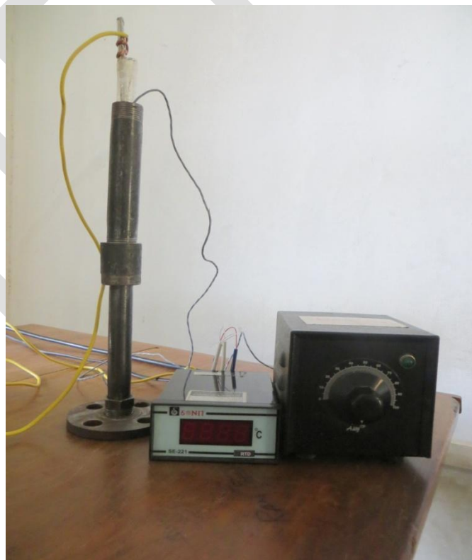
Fig:3.2 Transient hot wire thermal conductivity apparatus
