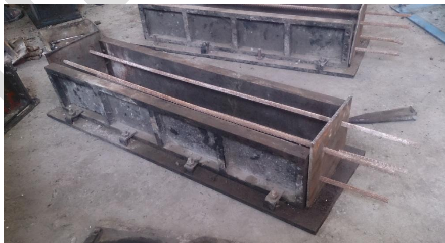
Fig.4 Prepared beam specimen with reinforcement
