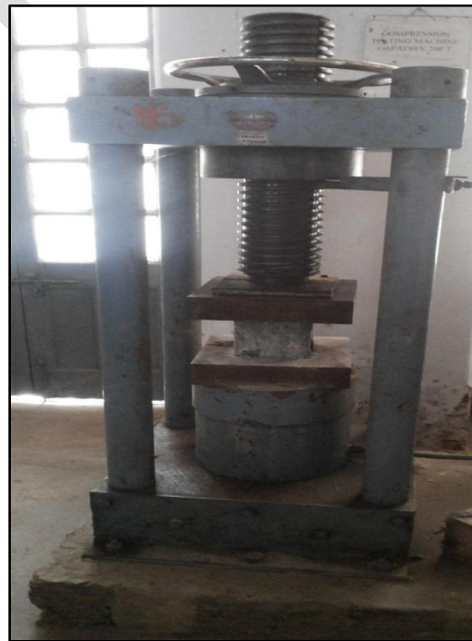
Fig.2 testing of cube specimen
