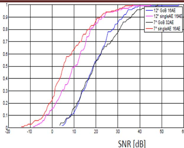
Fig.4. SNR for 90 users in single cooperation network
