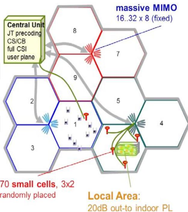
Fig.2. Details of overall multi layer system set up
