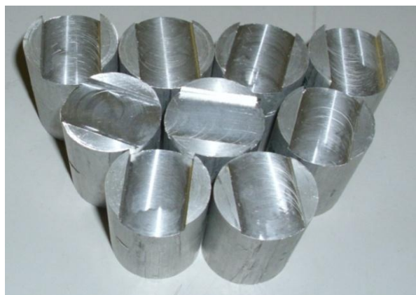
Fig. 1: (a) Milling of aluminium work piece; Fig.1 (b): Finished aluminium bars with single slot
