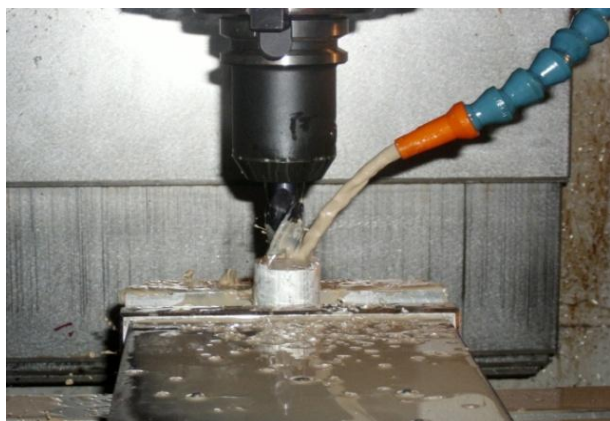
Fig. 1: (a) Milling of aluminium work piece; Fig.1 (b): Finished aluminium bars with single slot
