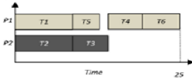
Fig 9: Schedule based on equal partitioned L2 cache
