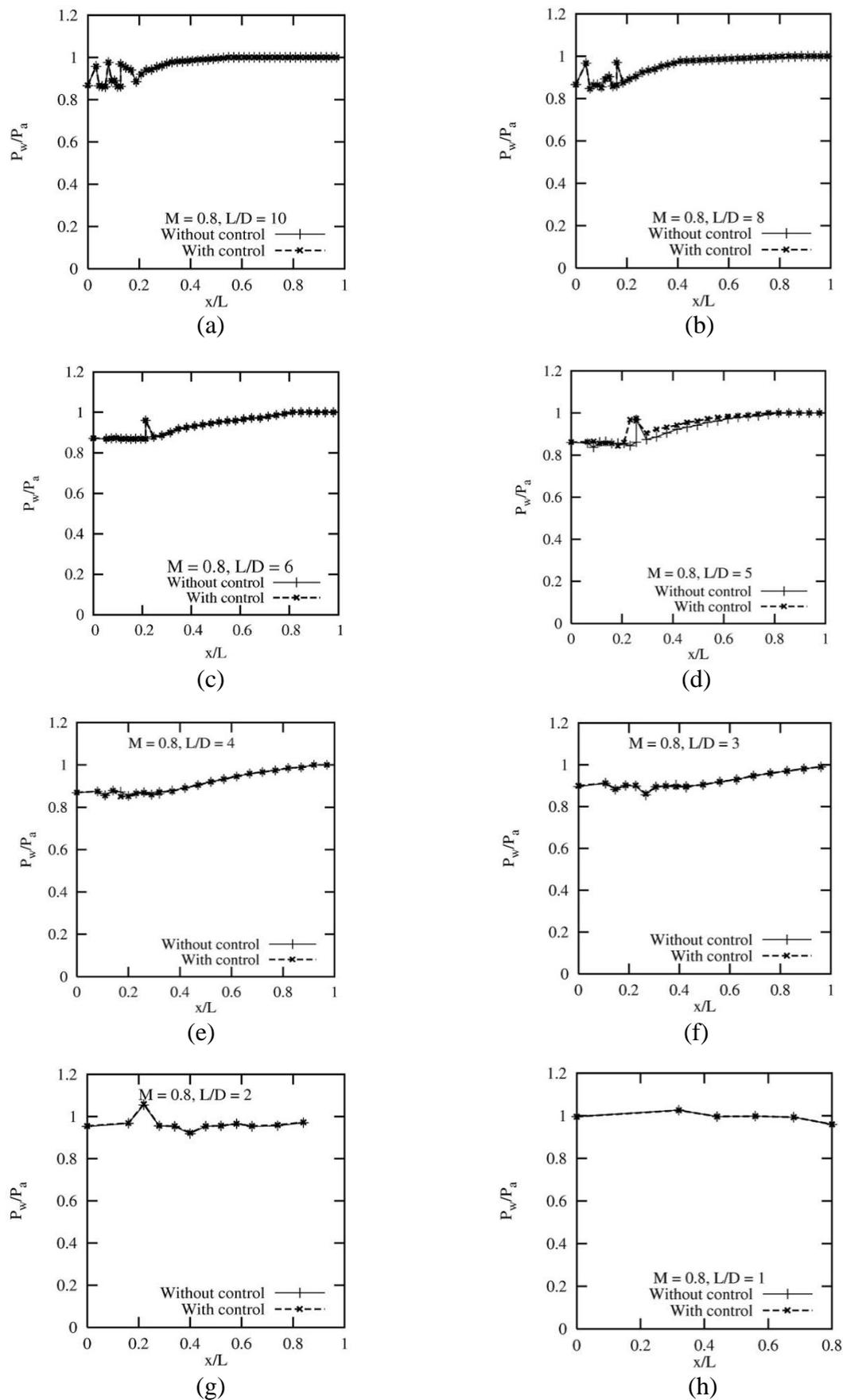
Fig. 3: Wall Pressure Distribution
