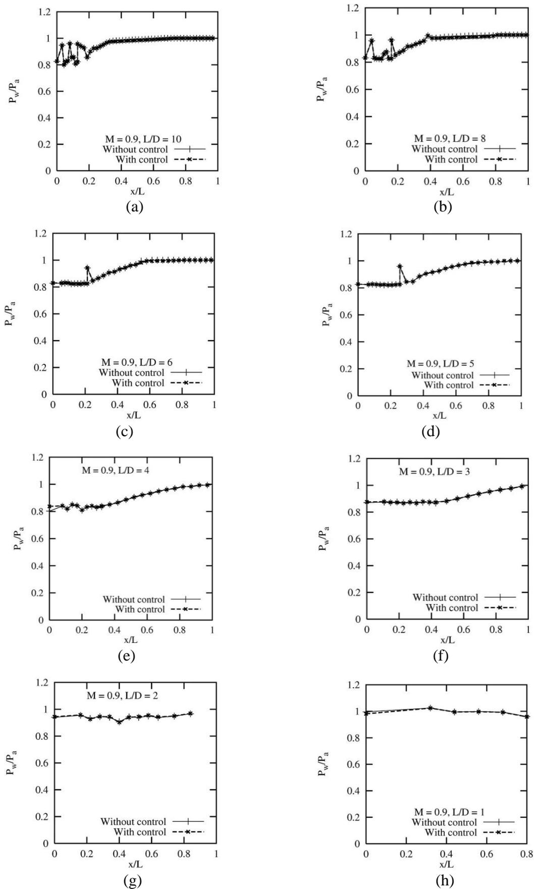
Fig. 2: Wall Pressure Distribution
