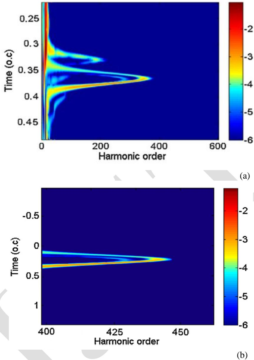
Fig. 3. The time–frequency distribution of the blue solid curve in Fig. 3 for  $a = 0.005$  and in the case of (a) linear inhomogeneous and (b) nonlinear inhomogeneous. (For interpretation of the references to color in this sentence, the reader is referred to the web version of the article.)
