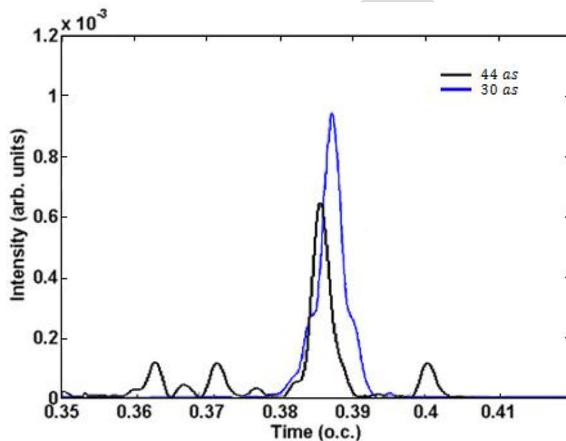
Fig. 2. (Color online) The isolated attosecond pulse in the linear inhomogeneous, for  $a = 0.005$  (black), obtained by superimposing 320<sup>th</sup>–420<sup>th</sup> order harmonics; this superposition resulted in a 44 attosecond pulse; in the case of the non-linear inhomogeneous,  $a = 0.005$  (blue), a 30 attosecond pulse was obtained by superimposing the 420<sup>th</sup>–487<sup>th</sup> harmonics.
