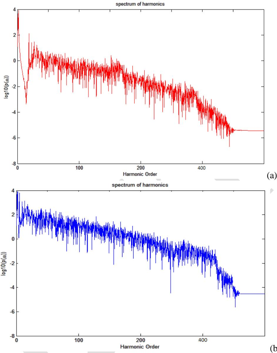
Fig. 1. (a) High-order harmonic generation (HHG) spectra for a He gas with  $E_{GS} = -0.58$  a.u. generated using the 1D\_TDSE. The laser parameters are  $I = 10^{13}$  and  $2 \times 10^{14} \text{ w/cm}^2$ ,  $\varphi_1 = \pi/2$ ,  $\varphi_2 = \pi/2$ , and  $\lambda = 800$  nm. We used a pulse with four optical cycles for  $a = 0.003$  (red) in linear inhomogeneous  $H(x)$  mode. (b)  $a = 0.003$  (red) in non-linear inhomogeneous  $H(x)$  mode.
