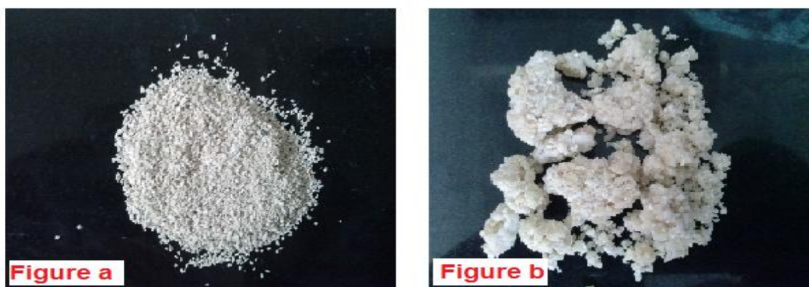
Figure 2. a. Crushed Waste Porcelain and b. Final adsorbing material
