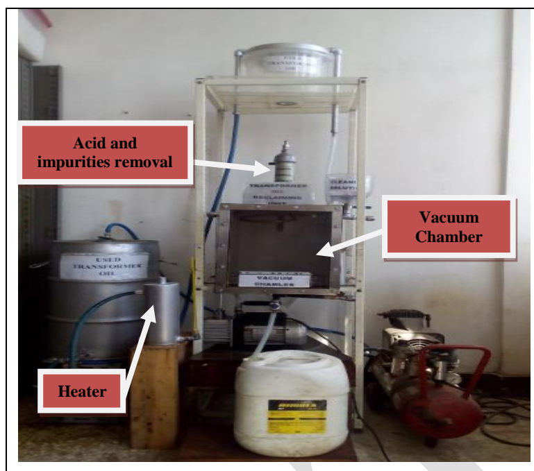
Figur(1): Typical photograph of the constructed refining unit.
