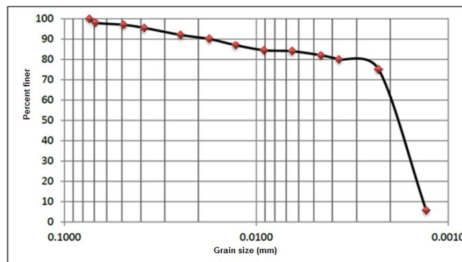
Figure 1: diagram of soil graining in hydrometer test
