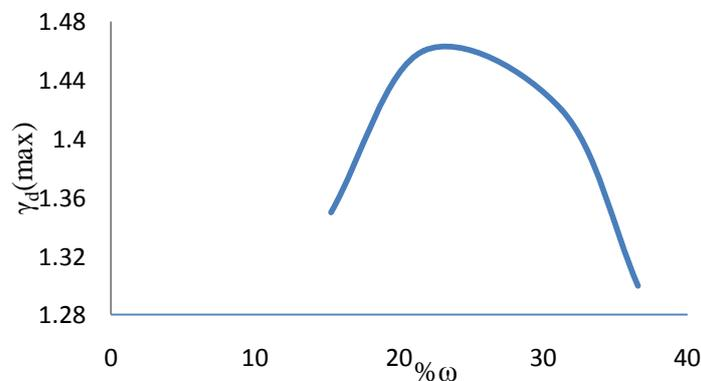
Figure 3: compaction test on primary soil
