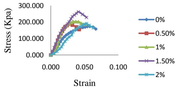
Figure 7:unconfined compression test for samples containing Nano-clay
