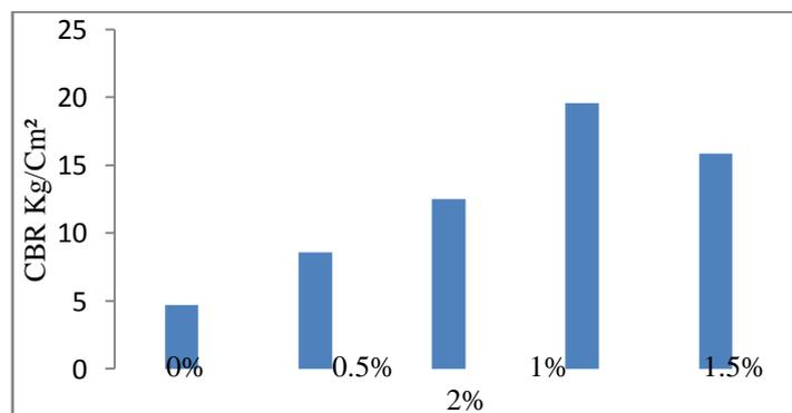
Figure 7:CBR test for samples containing Nano-clay
