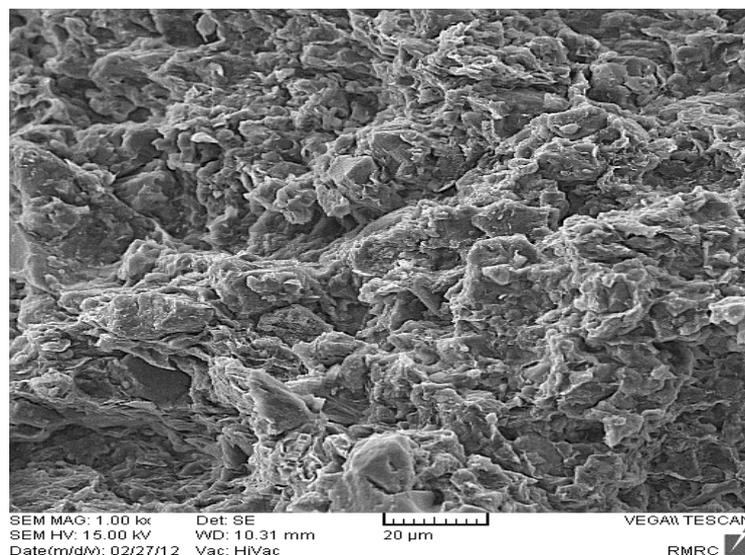
Figure 6: picture SEM from sample containing 2% Nano-clay
