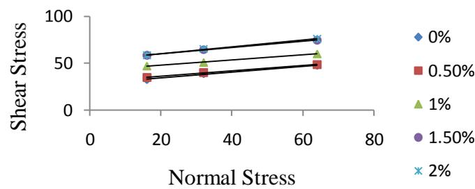
Figure 4: the process of shear strength in direct shear test. Cohesion increase in soil and being filled up of holes are clear in figure 5 and 6(SEM picture). As we can see in picture below Nano enhancement from 1 percent to 2 percent causes to fill holes within soli; so this being filled appears in shear strength .
