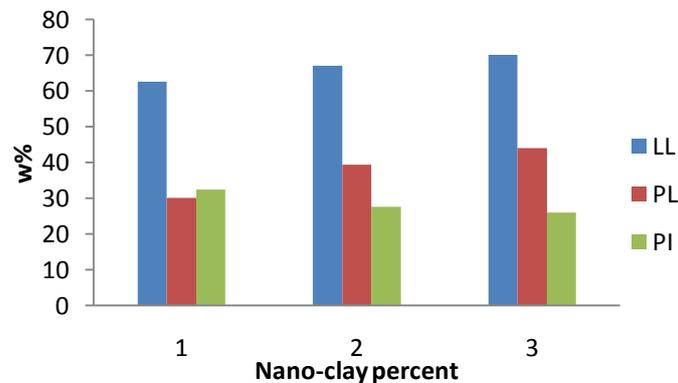
Figure 2: Atterberg limits (1, 2 and 3 in diagram respectively shows a 0% , 1% and 2% of Nano-clay)
