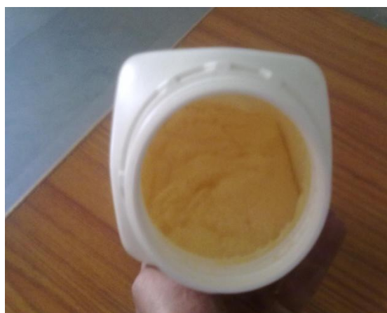
Fig. 2.1: Resin used for acid recovery
