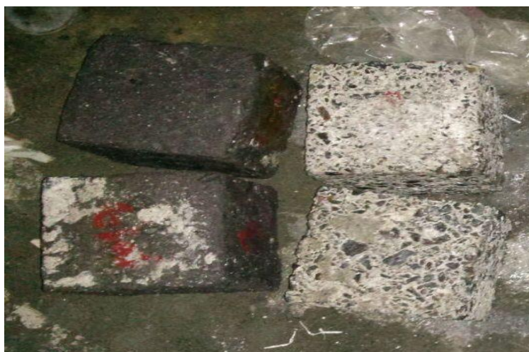
Photograph 3: Specimen cubes after acid attack
