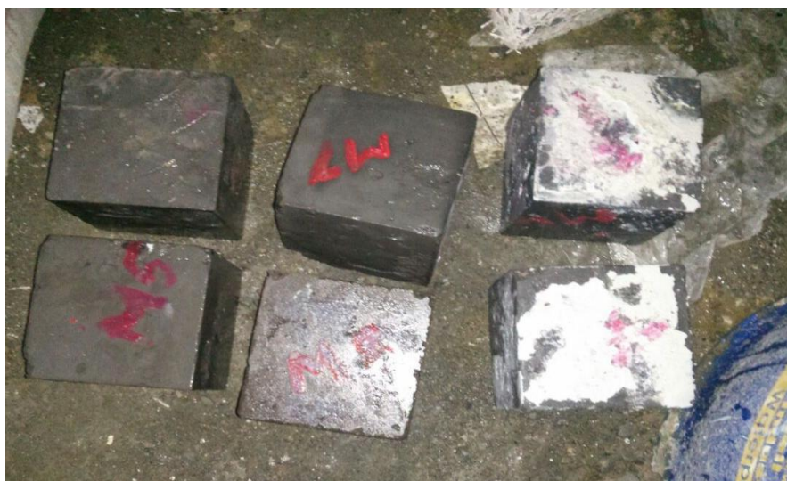
Photograph 4: Specimen cubes after sulphate attack
